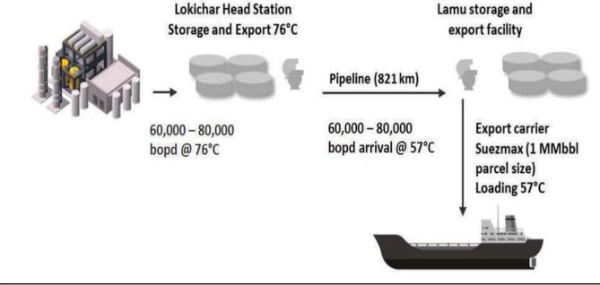
Figure 128: Upstream at Lokichar, Turkana; Midstream pipeline traversing through six counties of Turkana, Samburu, Isiolo, Meru, Garissa & Lamu; and Downstream distribution by the Suezmax carrier
