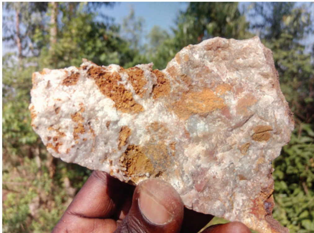
Plate 97: Gold-bearing quartz vein within the Archean Greenstones of Western Kenya (M. Nyakinye, 2023)
