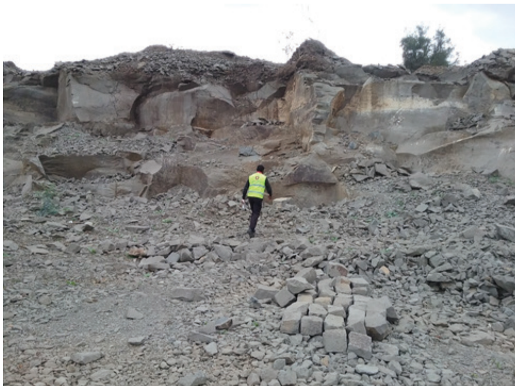
Plate 96: Tertiary volcanics being mined for aggregate and construction stone (M. Nyakinye, 2023)
